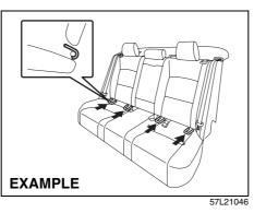
Your vehicle is equipped with lower anchors for securing up to one or two standard LATCH-type child restraint(s) in the rear seats. (LATCH stands for Lower Anchors and Tethers for Children.)
